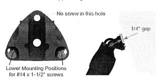
Pull the excess cable through the transom leaving enough cable to prevent the actuator from binding during its normal movement.
