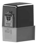
location to avoid submersion and drenching. Allow space above the HPU so that it may be slid into its mounting bracket (about 3"). Lay out upper holes on HPU mounting bracket 4-5/8" apart and start #10 x 1" screws using 5/32" pilot holes. Then drill 5/32" pilot holes for lower screws and secure bracket. Slide HPU into bracket.
