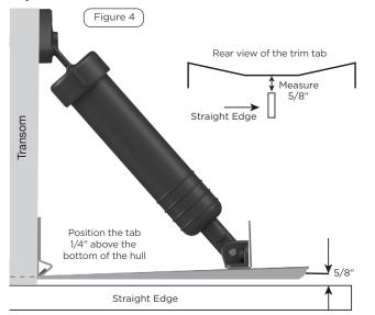
With tabs set at a 5/8" negative angle, position the upper mounts of the actuators against the transom. Slide the attached actuator template (see reverse page) behind upper mount, align and tape to transom. It is not necessary that the upper mounts lie flat against the transom as the
