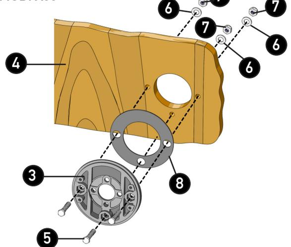
**Steering system assembly on the bracket**
