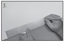
Mark the Pilot Holes. Using the same backing plate as a template, mark the pilot hole locations. Make sure the tabs can be mounted in the same location on both sides.
