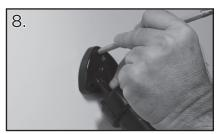
Mark Actuator Position on Transom. Set the actuator upper hinge against the transom. Mark the three upper hinge hole centers.
