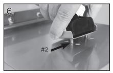
**Attach Actuator to Trim Tab.** Start with the center set of holes (Position #2), placing the mounting bracket in between actuator lower hinge and tab. Secure lower hinge with included 1/4-20 x <sup>3</sup>/<sub>4</sub>" Philips Head machine screws.
