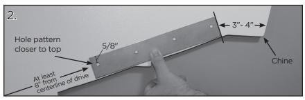
**Position the Tab.** Using the backing plate, choose a location 3-4" from the chine. Maintain a minimum of 8" from the centerline of your drive unit to the closest edge of the trim tab. Align the bottom of the backing plate flush with the bottom of the transom. The hole pattern on the backing plate should be closer to the top edge of the backing plate.
