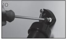
**Mount Actuator to Transom.** Apply marine sealant in and around pilot holes. Secure upper hinge to transom with #14 x 1 ½" screws.
