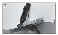
**Set Final Actuator Position.** Use a straight edge under the trim tab to make sure the tab is flush with the hull bottom. This is important to ensure correct actuator placement.
