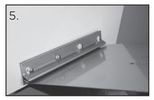
**Install Tab and Hinge Assembly.**Dip screws in marine sealant before inserting into pilot holes. Run the screws in 3/4 of their length. Slide trim tab between backing plate and hinge plate. Now, tighten the screws.
