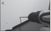
**Drill the Mounting Plate Holes,** using a 5/32" drill bit. (For aluminum boats, use #10-32 machine screws of an appropriate length instead of the screws supplied.)
