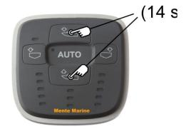
The AUTO indicator blinks to indicate that calibration is needed. Press the uppermost and lowermost buttons simultaneously for 5 s to start the calibration. Keep the buttons depressed for another 9 s, while the ACS is calibrating.
