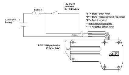
**Caution:** When wiring this two-speed motor as a single-speed you must use the slow speed as shown in the wiring diagram above and not the fast speed. Using slow speed will help to extend the life of the motor.
