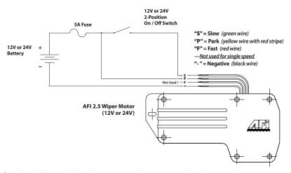
**Caution:** When wiring this two-speed motor as a single-speed you must use the slow speed as shown in the wiring diagram above and not the fast speed. Using slow speed will help to extend the life of the motor.
