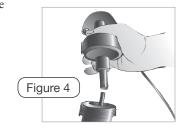
Tighten the upper hinge hand tight. You will finish tightening the cylinder in Step 7.
