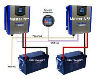
**Example 3**: Case of the 24V100A model (battery charger with 2 power PCB)
