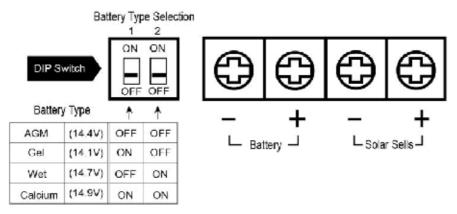
Figure 1.1: Battery Type Setting via DIP switch
