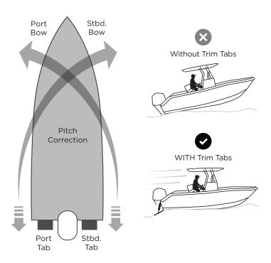
When the tabs are deployed downward, the water force on the trim tab surface creates upward pressure, raising the stern and lowering the bow. The port trim tab lowers the starboard side bow, and the starboard trim tab lowers the port side bow.
