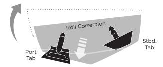
When the port tab is lowered independently, an upward force at the port stern of the boat is created. The inverse applies when lowering the starboard tab independently.
