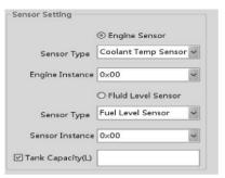
In product option, to select sensor enter sensor parameter setting; select engine sensor/fluid level sensor per product's type.
