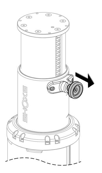
A spring-loaded knob located on the side of the pedestal retracts the locking pin, allowing the seat to be raised or lowered.
