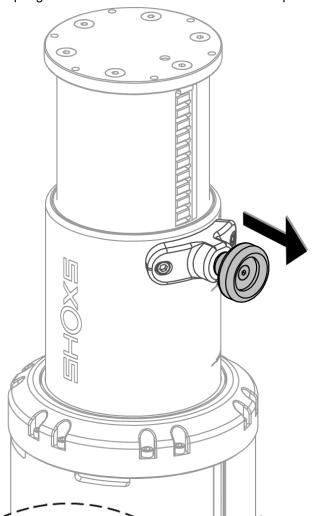
While in a standing position, pull the knob and adjust the seat to the desired height. The pedestal may not rise on its own, depending on the weight of the seat and components installed.
