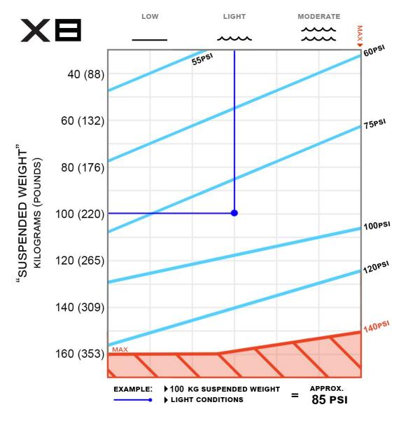
THE PRESSURES INDICATED IN THE TABLE ABOVE ARE RECOMMENDATIONS ONLY. THE RESULTS OF TESTING IN ACTUAL CONDITIONS USING THE **STATIC LIMIT** AND **OPERATING LIMIT** INDICATORS ARE THE FINAL DECISIVE FACTORS IN WHICH PRESSURE TO USE IN SERVICING AND OPERATING YOUR SHOCK MITIGATING PEDESTAL. ALWAYS ERR TOWARDS A HIGHER PRESSURE TO ENSURE PROTECTION FROM 'BOTTOMING' THE ISOLATOR'
