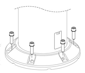
Note: Preferred installation orientation is with the **side access door** of the pedestal facing **aft**. SHOXS logos on the upper pedestal will be on the STBD and PORT sides of the unit.
