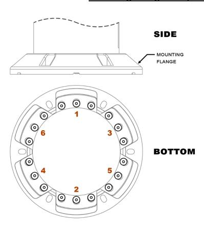
The **mounting flange** of your shock mitigating pedestal is shipped installed in the lowest position available. This torque procedure **must be followed** if loosening the fasteners to adjust the position of the mounting flange.
