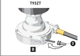
6 Insert bushing (3) completely and lock it by means of screw (4). Torque: 6 Nm (53 inch lbs).
