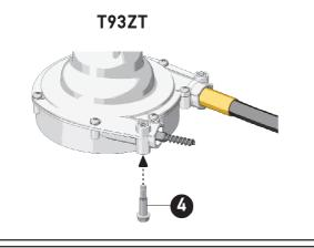
7 Insert protection pipe (5) on bushing (3).
